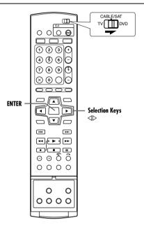
If you have connected the unit to your TV via a 21-pin SCART cable (pg. 18), the unit will automatically perform Preset Download instead of the Auto Set Up in step 2 on page 19. After downloading, the unit sets the clock and Guide Programme numbers automatically.
